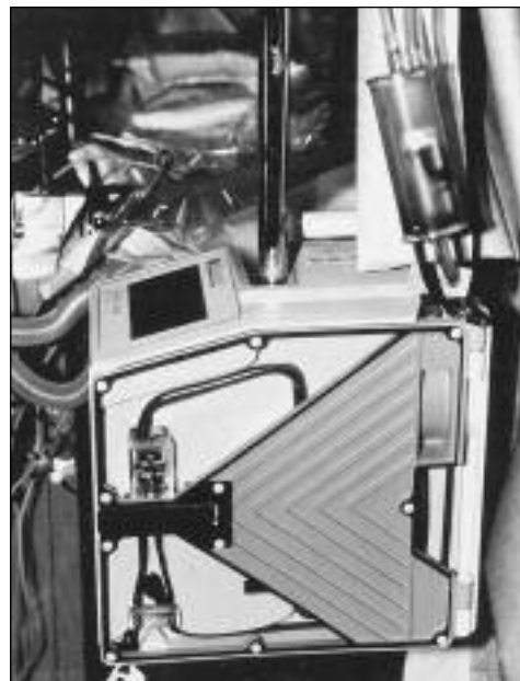
Figure 2. Belmont FMS 2000 warming system (Belmont Instrument Corp., Bellerica, MA). The system consists of an integrated volumetric infusion pump coupled with a high-capacity magnetic induction heater. There are two ultrasonic air detectors, one at the fluid inlet and the other at the outflow to the patient coupled to an automatic shut off.
