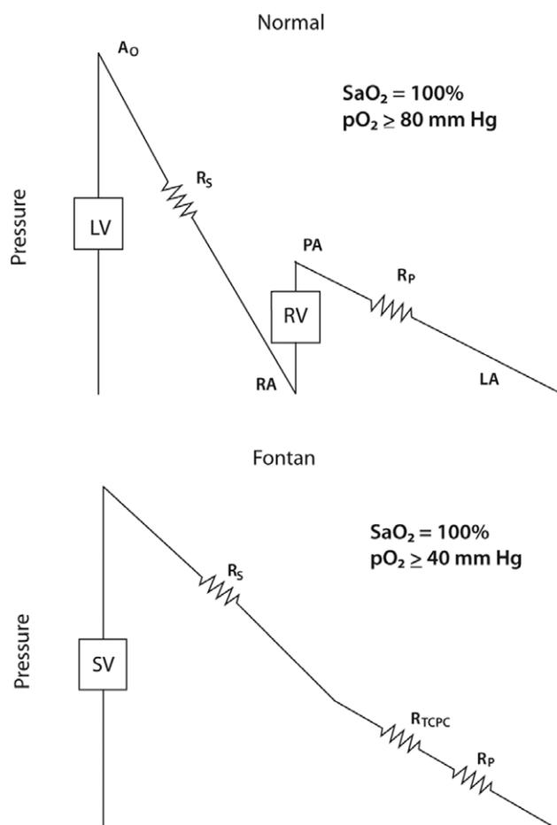
**Figure 3.** Schematic of the normal and Fontan circulation demonstrating a single-ventricle driving flow across 3 resistances in series; systemic ( $R_s$ ), total cavopulmonary connection ( $R_{TCP}$ ), and pulmonary ( $R_p$ ). In a normal, 2 ventricle circulation, each ventricle drives flow across 1 resistance (Adapted from Rodefeld et al.<sup>22</sup> by Katherine Black).
