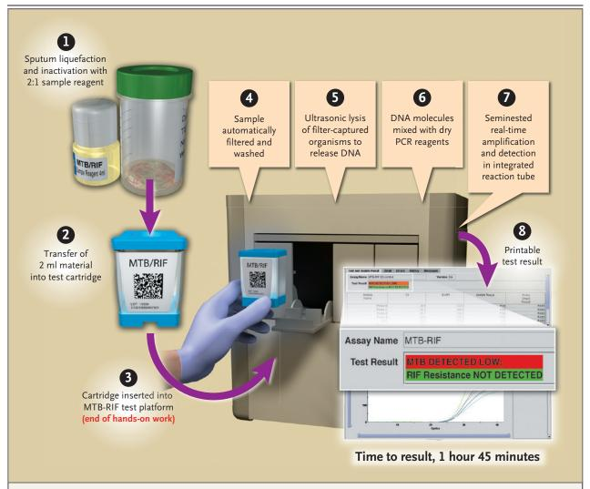
Figure 2. Assay Procedure for the MTB/RIF Test.
