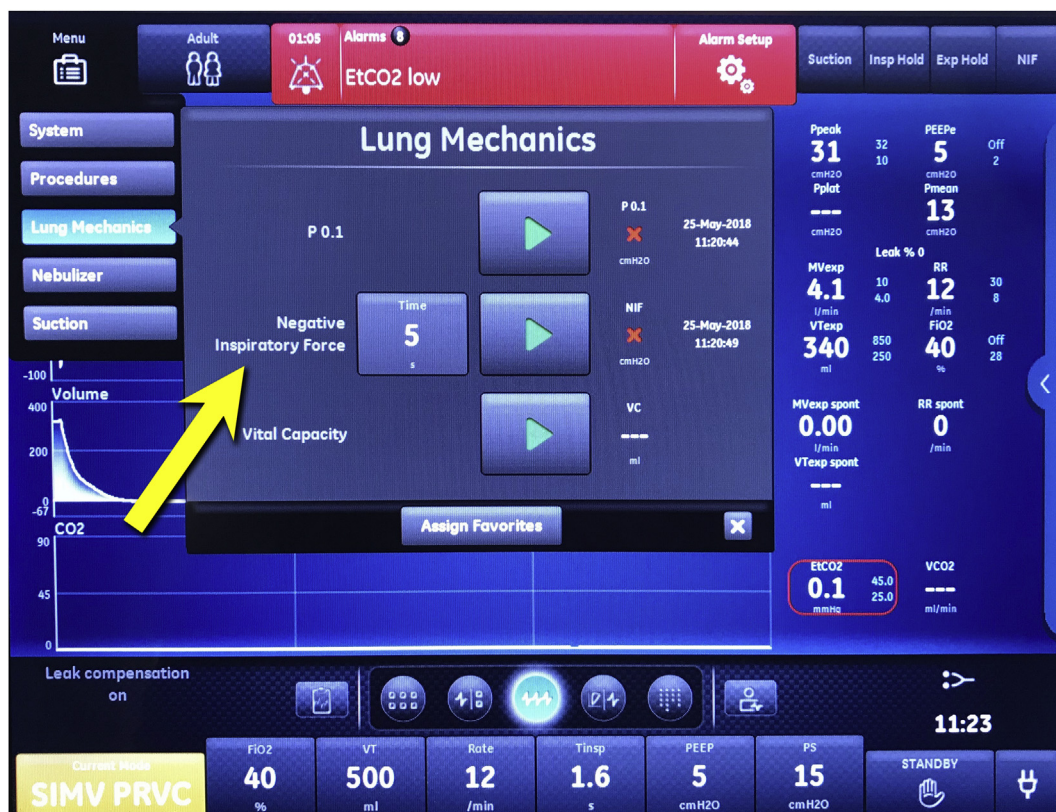
Fig. 5. Negative inspiratory force (NIF) measurement through the ventilator.
