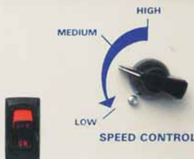
FIGURE 7 The flow rate on this machine is adjusted with the dial on the right-hand side.
