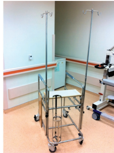
Figure 2. Custom-made walker for ventilated patients. The walker incorporates a walking frame on wheels, intravenous pole, oxygen basket and platform to support a ventilator, all in a single device.
