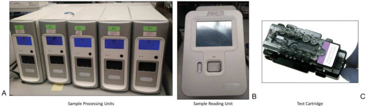
Fig. 3 The Nanosphere Verigene System, consisting of instrumentation (A, B) and the test cartridge (C). Sample and reagents are added to the processing unit. After analysis is completed, the cartridge is moved briefly to the reading unit for interpretation.
