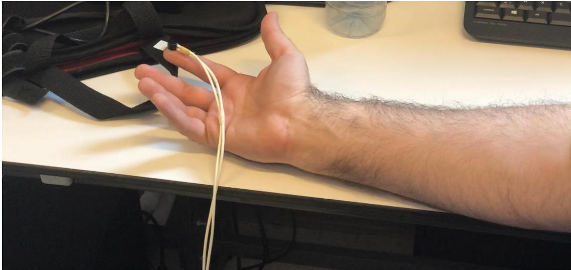
Figure S1. Thermostatic skin laser Doppler (SLD) probe (Reference number 457, Perimed, Jarfalla, Sweden)
