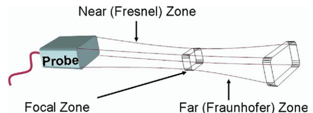
**Fig 11.** Characteristics of an ultrasound beam. The focal zone is where the ultrasound beam width is narrowest and demarcates the near zone (Fresnel zone) from the far zone (Fraunhofer zone). It is also the area of the best lateral resolution because the beam width is the narrowest at this location. Once the beam extends beyond the focal zone, lateral resolution begins to deteriorate due to divergence. This figure represents a prototypical electronically-focused ultrasound beam.
