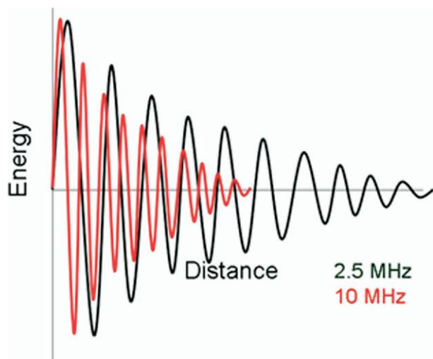
**Fig 7.** Attenuation. Attenuation is estimated as  $\alpha \times f \times$  path length, where  $f$  is the frequency of the ultrasound wave and  $\alpha$  is the attenuation coefficient. Notice the lower frequency wave (2.5 MHz) has less attenuation at a given distance when compared with the 10 MHz wave. Thus, the 2.5 MHz wave is able to penetrate the tissue more effectively than the 10 MHz wave.
