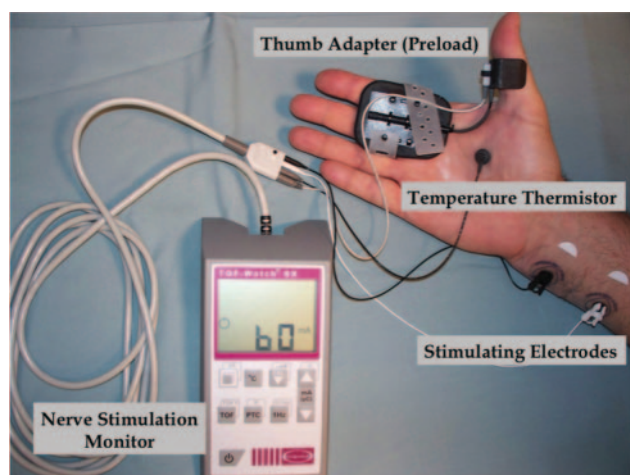
Figure 4. Example of acceleromyograph (AMG). The thumb movement in response to ulnar nerve stimulation is sensed by the piezoelectric sensor that is fixed to the thumb via the thumb adapter, and the acceleration (which is proportional to the force of muscle contraction) is sensed by the interfaced monitor. The current amplitude is displayed by the AMG monitor (60 mA on the screen). To improve the consistency of responses, the piezoelectric sensor is fixed to the thumb, which is placed under slight tension (200–300 g, “preload”) by the thumb adapter.
