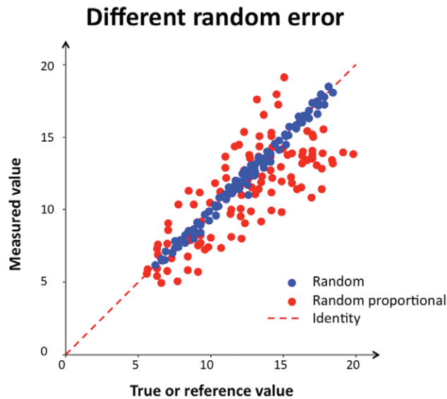
Figure 2. Schematic representation of 2 types of random errors. Blue plots, small random error ( 2\sigma = 0.6 ) typically seen when an independent noise is properly filtered. In red plots, the variability in proportion to the measurement value indicating that the random noise is getting into the signal. In these examples, both data sets have correlation slopes on the identity line (black dotted line), indicating no systematic errors (x-axis and y-axis with arbitrary units).
