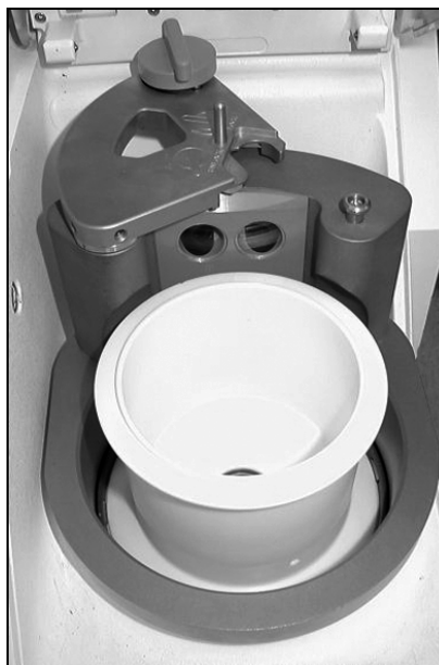
Figure 4-7, Inserting the chuck adapter (for use with the 70mL Bowl)
