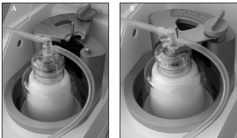
Figure 4-8, Securing the centrifuge bowl (steps A and B)
