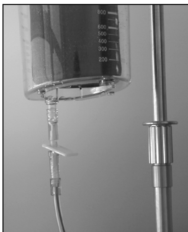
Figure 4-15, Connecting the red line to the reservoir
