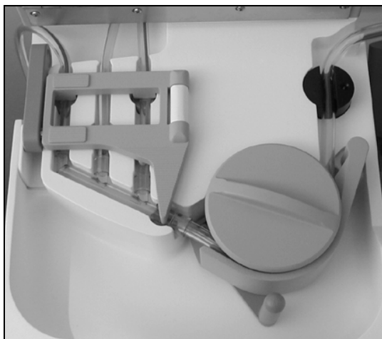
Figure 4-10, Securing the tubing harness
