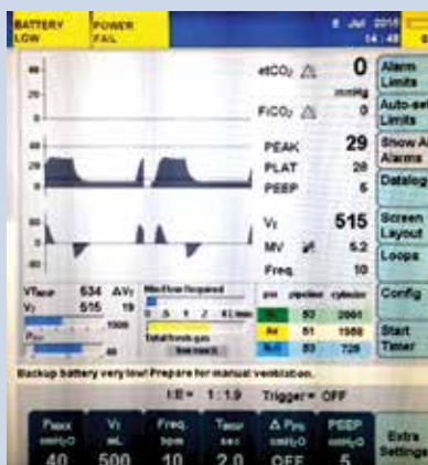
Figure 1. Screens displayed on Dräger Apollo and Fabius GS anesthesia machines at time of battery failure.
